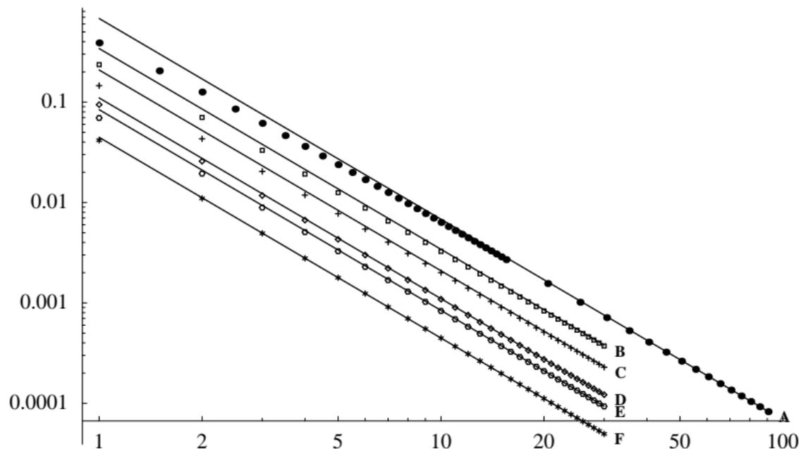
The **points** show the numerical evaluation of six different  $10j$  symbols as the scale factor  $\lambda$  ( $x$ -axis) is varied. The **lines** show the asymptotic predictions using degenerate points.
